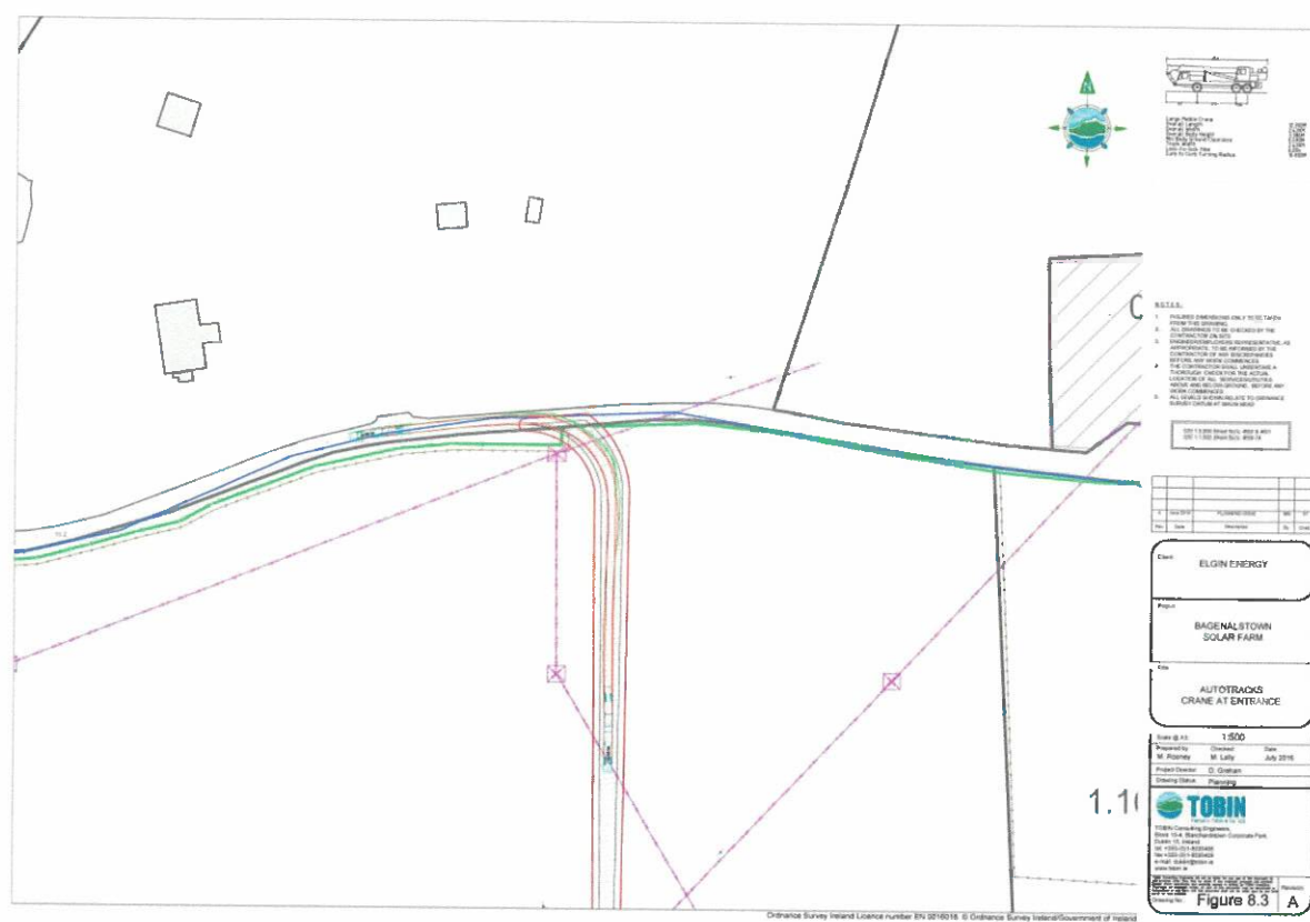
Figure 8.3 Autotrack Assessment Entrance – Crane
