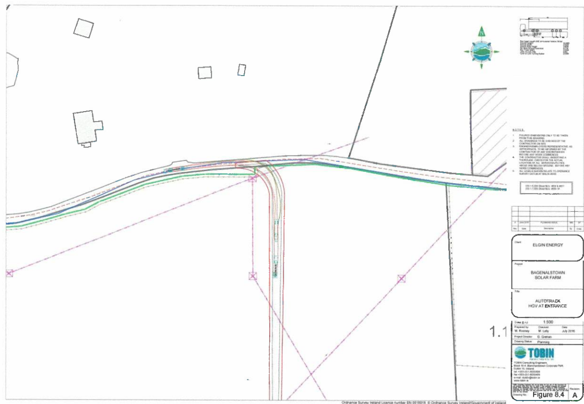
Figure 8.4 Autotrack Assessment Entrance - HGV
