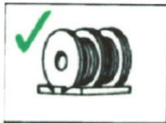
Figure 2 Storage of cables.
